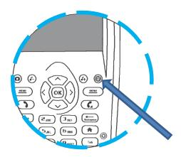
Press and hold the power button for 2 to 3 seconds, the power indicator will light on automatically, and at the same time, the startup picture will be displaying on the screen.
